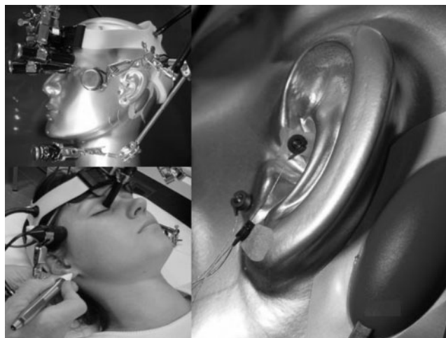
Figure 2: P-STIM® electrical point stimulation system and probe holder construction for the experimental transcranial ultrasound spectroscopic and near infrared spectroscopic investigations
